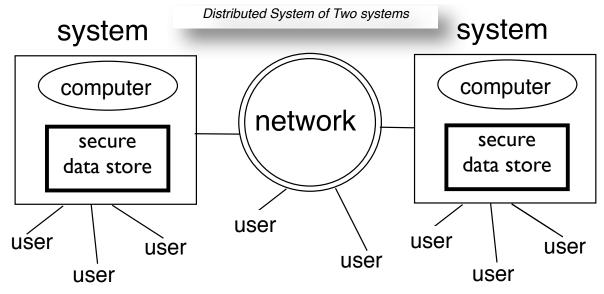
The schematic diagram above illustrates how two or more systems combine with a network to create a distributed system. Right away we see that the distributed information system has multiple management control areas - a potential issue - and an information sharing problem. How can a user on one system take advantage of information stored on another problem?
